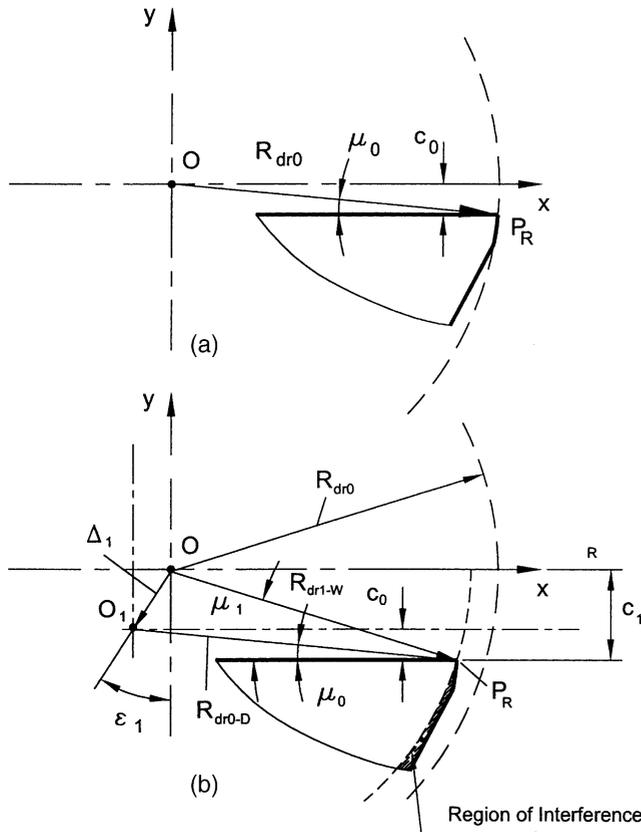
Fig. 10. The displacement of the drill periphery point  $P_R$  after the first stage of drill entrance.
