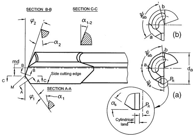
Fig. 2. Gundrill geometry.
