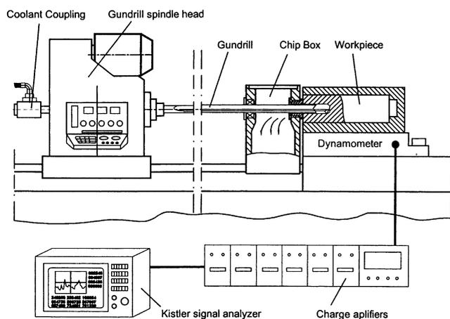
Fig. 4. Schematic of the experimental setup.
