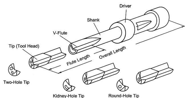
Fig. 1. Typical gundrill.
