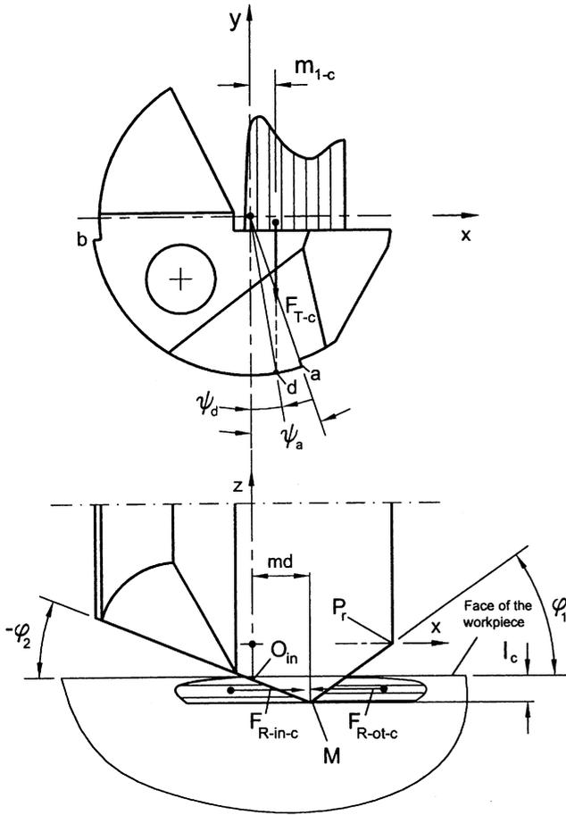
Fig. 7. Force distribution at the end of the first phase.
