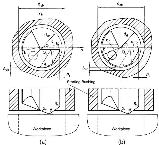
Fig. 6. Initial position of the gundrill in the starting bush. (a) Gundrill having supporting continuum  $ab$ . (b) Gundrill having two supporting pads  $a$  and  $b$ .
