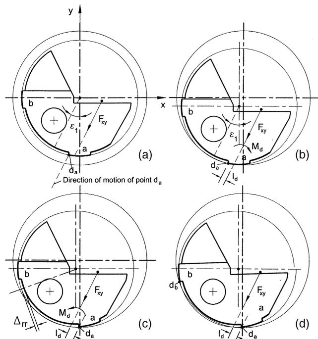
Fig. 11. Position of a drill having two supporting pads in the starting bushing after the first stage of drill entrance.
