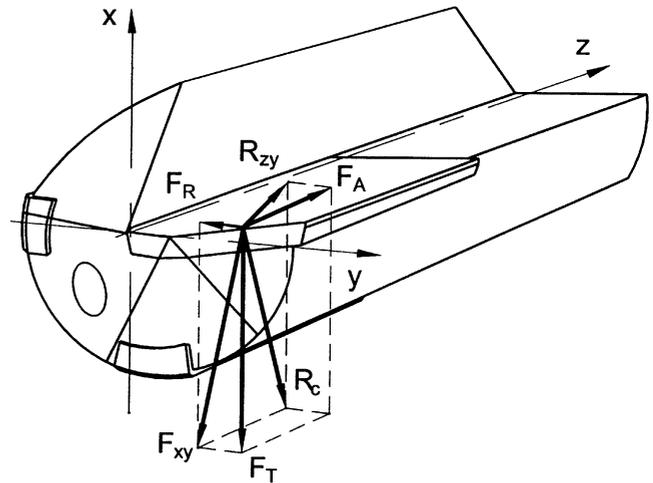
Fig. 3. The system of forces acting in gundrilling.
