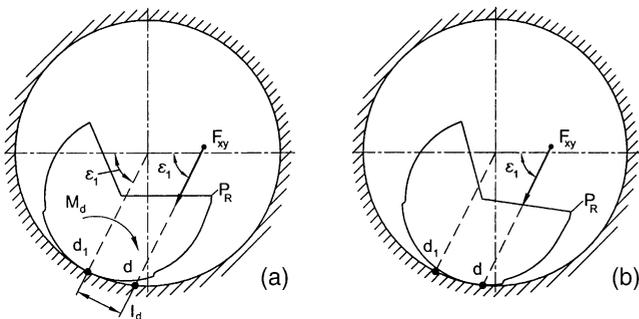
Fig. 9. The additional tilting moment  $M_d$  as an inherent feature of any gundrill having the supporting continuum.
