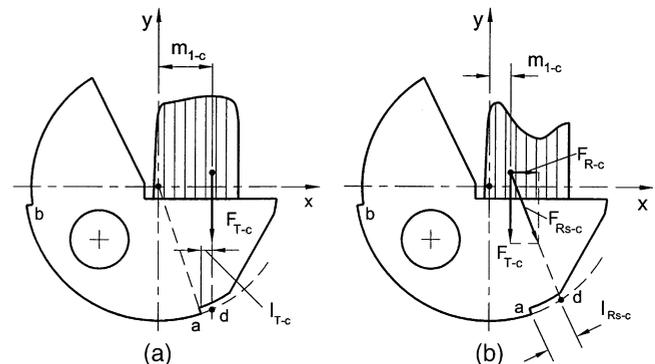
Fig. 8. The location of point  $d$  defines drill's stability at the entrance.
